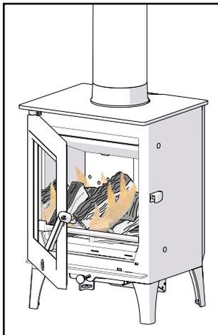
**Once kindling is alight, add smaller logs.** Keep air control fully out and close door.
