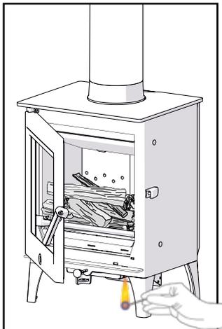
**Add kindling and paper or firelighters.** Keep air control fully out and door cracked open.
