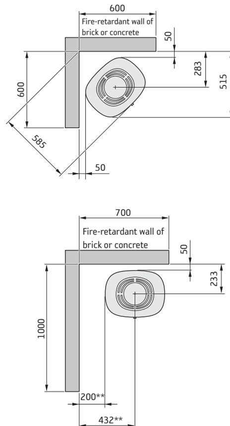
\* If the stove is placed on a hearth plate made of glass for example (accessory), the height from the floor is affected by a distance corresponding to the thickness of the hearth plate, for a free standing glass hearth plate this is 10 mm.
