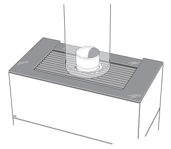
Supply of combustion must be provided. Combustion air can be provided directly via a duct from outside, or indirectly via a vent in the outer wall of the room where the stove is placed. The amount of combustion air that is used for combustion is approx. 25 m<sup>3</sup>/h. Some installation alternatives are shown to the right. The air duct connection on the stove has an external diameter of  $\emptyset$ 100 mm.
