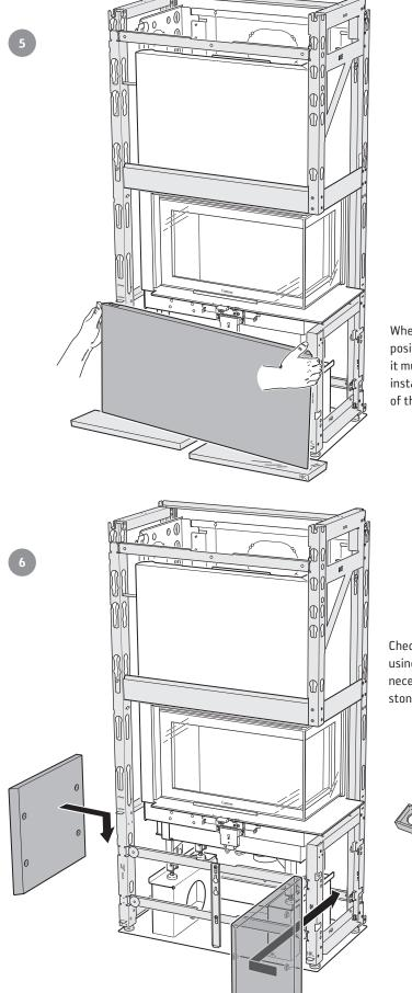
When the front panel is correctly positioned in the depth direction, it must be lowered again for the installation of the side panels. Beware of the corners!
