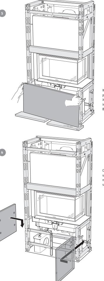
When the front panel is correctly positioned in the depth direction, it must be lowered again for the installation of the side panels. Beware of the corners!
