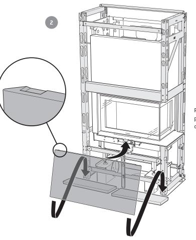
Place a foam sheet on the floor to prevent the stone corners from becoming damaged when handling.
