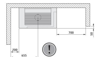
For placement against combustible rear walls, a builtin protective screen (option in some markets), or an external firewall that protects the wall behind is required. Material requirements for firewalls according to the section "Walls behind" on page 228.
