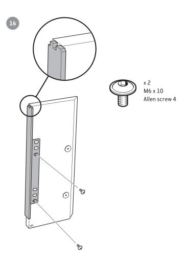
The front panel must rest on the stand's metal tab, not on the lower front In the event of having to insert shims, do this on the metal tab.
