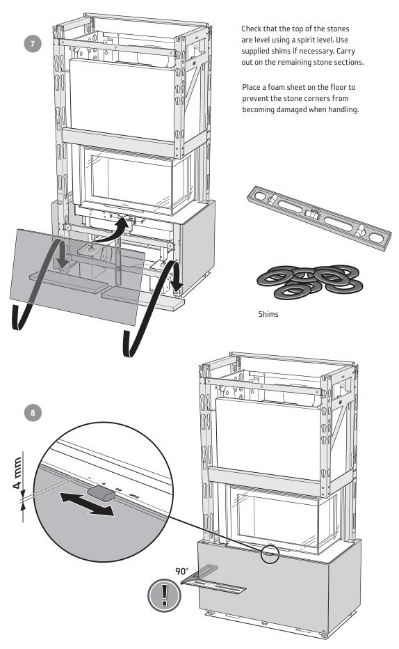
Ensure that there is a 4 mm gap between the stone and insert so that the damper can move freely.
