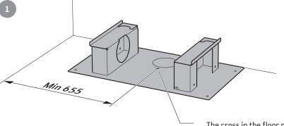
The cross in the floor panel indicates the location of the flue gas output.
