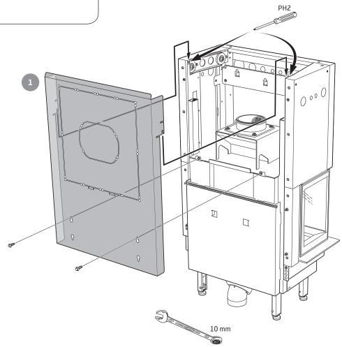
Position the floor section and check that the minimum permitted distance to combustible material is kept. Measure to the centre of the floor section.
