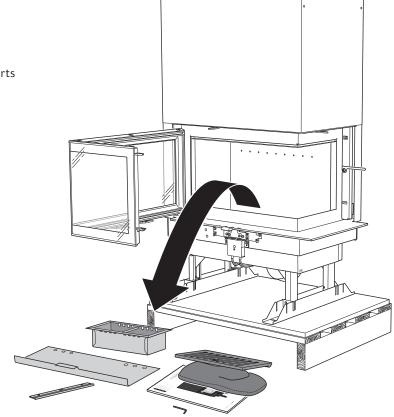
The insert is secured to the pallet by the two rails, remove the screws and remove the angle brackets. Reinstall the screws on the legs before moving the insert from the pallet.
