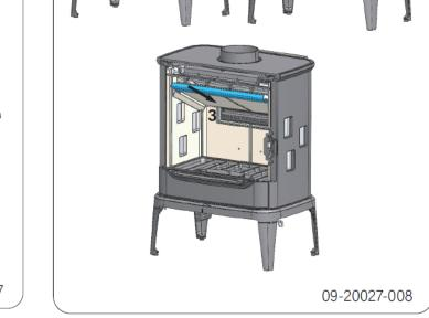
Order of inserting stainless steel baffle plates:
