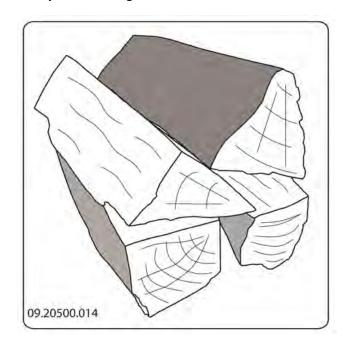
If the logs are stacked tightly, the wood will burn more slowly as the oxygen can only reach some logs easily. If you want to burn wood for a longer period, make a compact stack.
